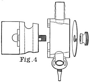
Figure 4 shows the parts of the three-way-cock separated: on the left the plug of the stop-cock, next to this the shell, and on the right a disc and thumb-screw for holding the plug in place.
